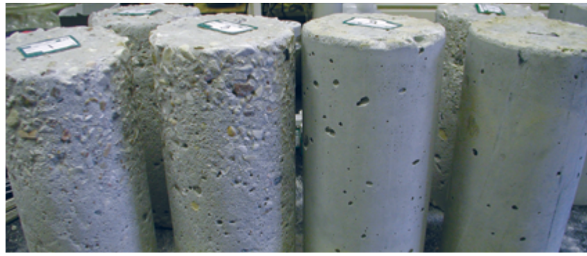
Figure 1: Concrete cylinders after 30-day test with BoviBrom (DBDMH)
