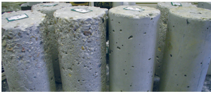
Figure 1: Concrete cylinders after 30-day test with AviBrom (DBDMH)
